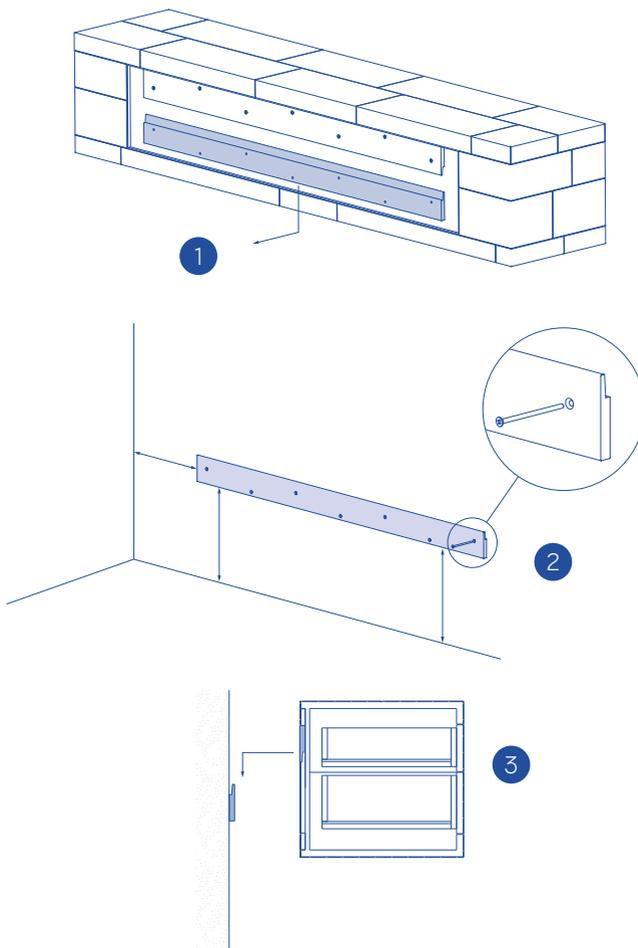
Remove the bracket from the console (fig. 1). Secure the bracket to the wall using the most appropriate anchoring system for the wall type (fig. 2), ensuring it is properly aligned using a level. Hook the cabinet onto the bracket (fig. 3). De Castelli declines all responsibility for any damage or malfunction resulting from the incorrect choice of wall-fixing method.
